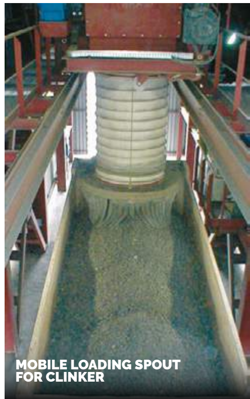
CAPACITY: 250 ton/h STROKE: 5.200 mm
